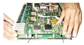
Fig 3.5.2e Daughter Bd. Being placed over the Grand daughter Bd. and the mating connector being matched to lockup properly Step 4. Hold the daughter board with both hands at the end and align the two cream
